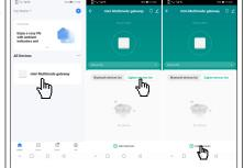
6. Press and hold Test/mute button after the led light is ON about 10s, led will flash quickly, loose the button while the buzzer sound "Di" once, device get into internet connection status, wait the APP get into the "device searching" interface, and search the "smoke alarm detector" and add the device succeed.
