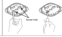
3.Refer the image as below, Interpoint the product body with the bracket, rotate the product body clockwise, and
